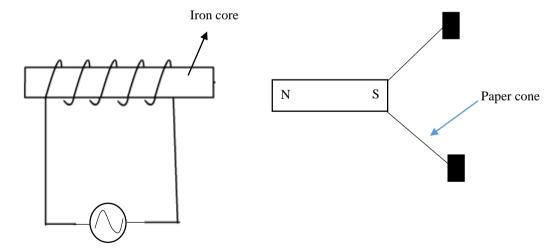
When the battery is replaced with an a.c. source, the polarity of the coil will keep reversing repeatedly. This will cause the bar magnet to move towards and away from the iron core repeatedly as it keeps getting attracted and repelled in quick successions. This causes the paper cone to vibrate and produce longitudinal sound waves.
