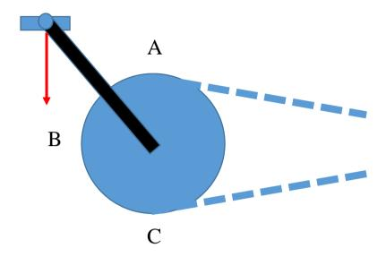
When the pedal is at A, no moment is produced as there is zero perpendicular distance between the pivot and the pedal at A.
