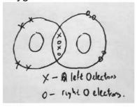
ii) For magnesium oxide, magnesium loses two electrons, forming Mg<sup>2+</sup> ion, while oxygen gains those two electrons to form O<sup>2-</sup> ion. For oxygen molecule, the two atoms of oxygen share two sets of electrons to form a strong double bond.
